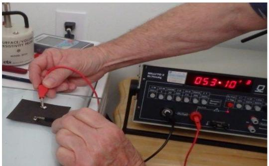
Mercury reading = 5.3E3 Ohms
