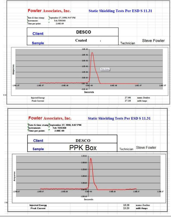
To make the difference more obvious, a 10 kV HBM discharge was presented to the top of each box with the electrode inside near the inside top of
