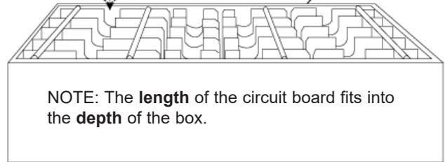
In measuring a circuit board, you must be aware of any components or leads that extend past the board. These extended parts could be damaged if loaded into the cell and placed at the bottom of the In-Plant Handler. Therefore, make sure that the width dimension has no protrusions. If your board has protrusions, then reverse the length and width dimensions to make sure your board fits properly in the In-Plant Handler. When in doubt, send us a sample of your circuit board.
